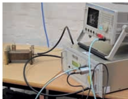
TMD's PTC6441 amplifier (bottom unit) in use for the 'MICROGRASS' project.
